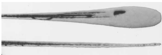
Fig. 2. Crevice corrosion in a PWR component after a burnup of 52 MWd/kgU.
